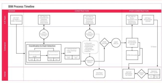
BIM Execution Plan During Design-to-Engineering-to-Construction Process
